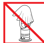
In order to avoid overheating and fire hazard, do not cover the heater.
